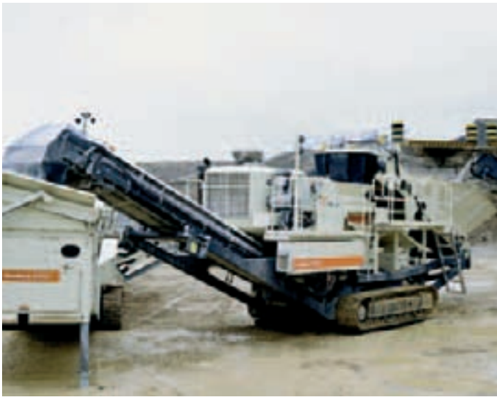
Lokotrack LT200HP can be easily operated with a primary impactor or jaw plant and with a mobile screen.
