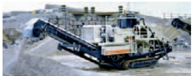
Lokotrack LT200HP cone plant.
