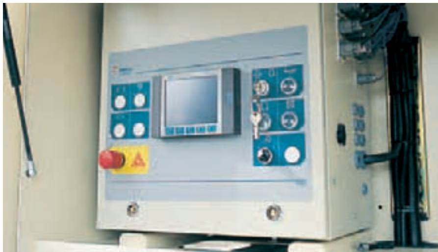
The revolutionary IC700 intelligent controller controls the whole crushing operation and gives real time crushing information about all the main functions.
