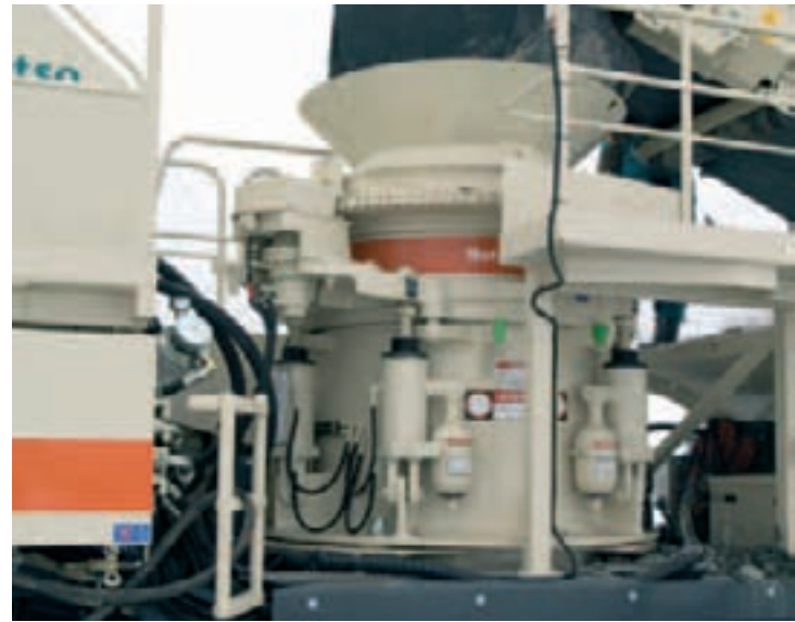
LT200HP is built around the proven and popular HP200 cone crusher.
