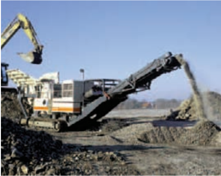
The sturdy and long main conveyor can be equipped with an optional magnetic separator for recycle applications.
