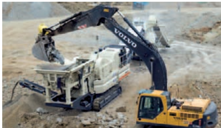
LT116 in a two stage crushing and screening process with LT200HPS cone plant.
