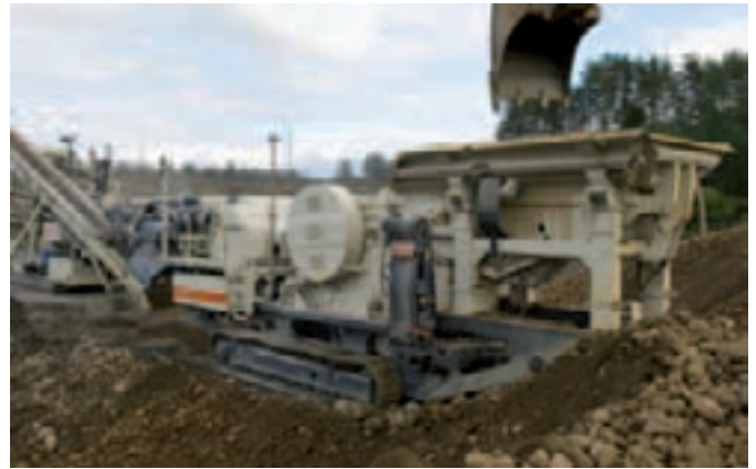
Lokotrack LT116 feeding a LT1100 cone plant.
