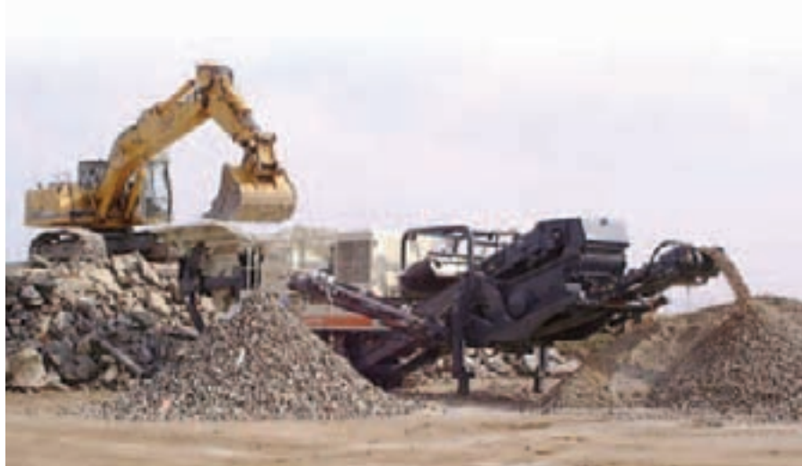
The Lokotrack LT96S crushing recycled concrete in Germany.
