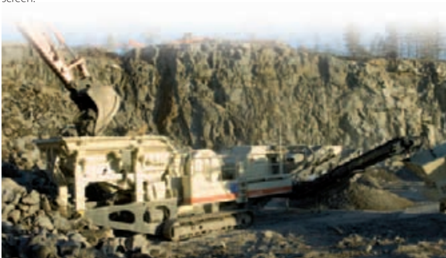
The screening unit can be disconnected in minutes allowing the Lokotrack LT106S to be used as a normal primary crushing unit.
