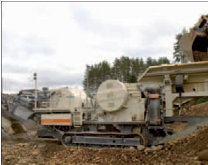
LT116 crushing natural gravel in Finland.
