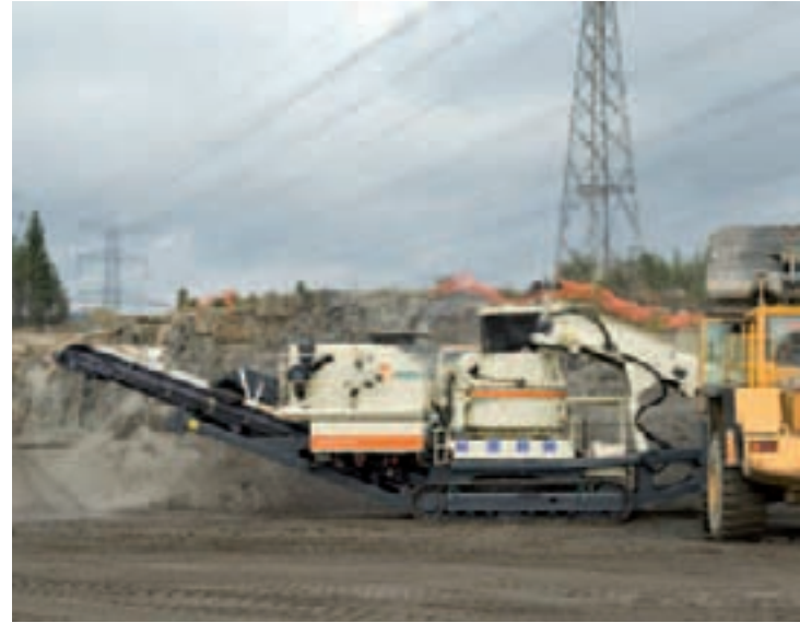
Thanks to the large feed hopper, LT7150 can be fed with conveyor, excavator or wheel loader.
