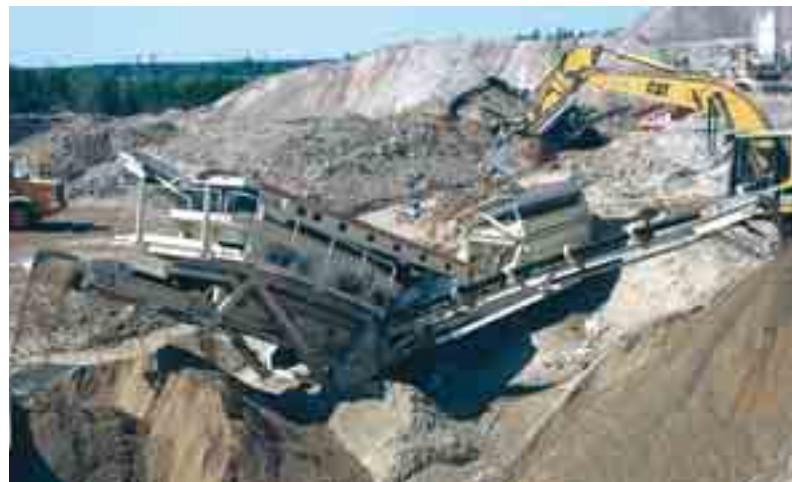
The Lokotrack ST352 is available with a direct feed system when hopper and feed conveyors are not needed.
