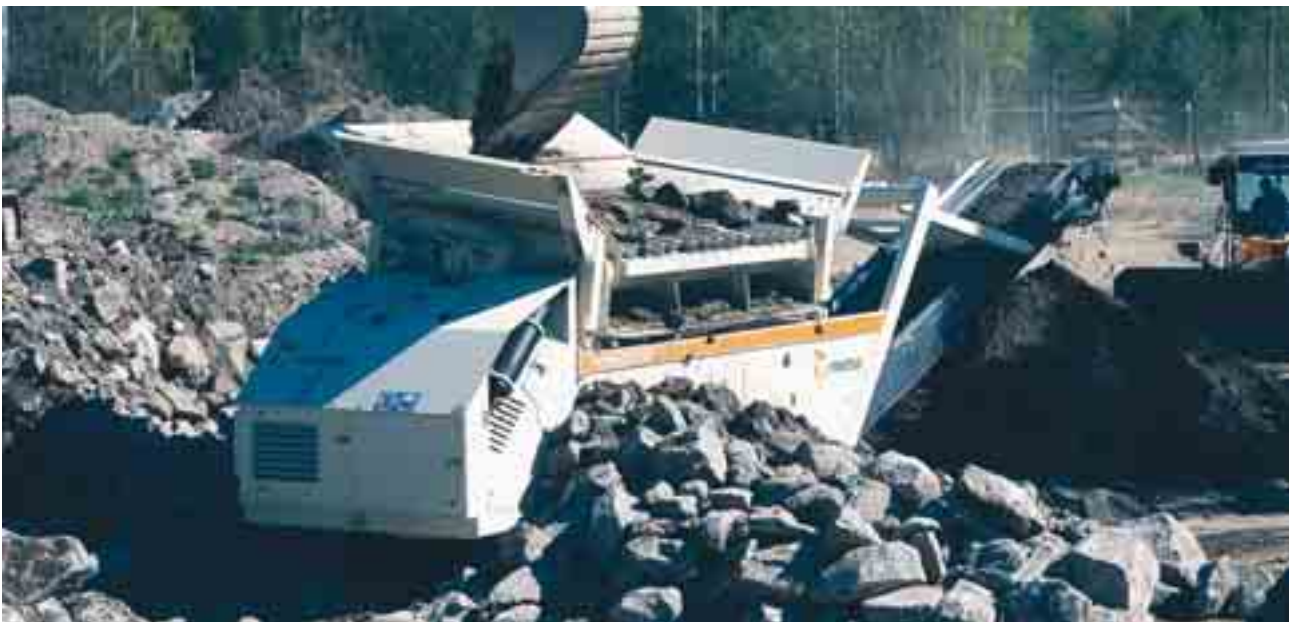
The forward and reverse shakerhead motion of Lokotrack ST71 mobile screen allows to obtain maximum screening efficiency with difficult materials.
