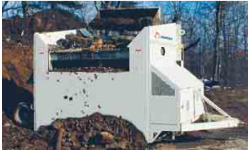
Woven screen cloth, punch plate, harp screens or finger decks can be used with Nordberg CV50's patented, convertible shakerhead.
