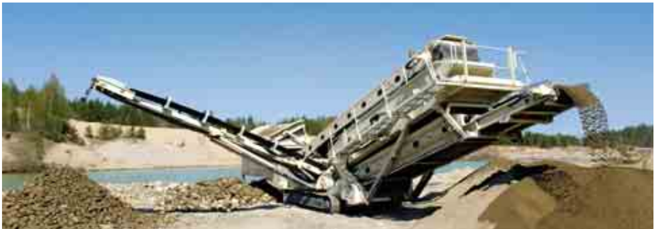
Lokotrack ST358 mobile screen features large capacity hopper and extra wide product conveyors.
