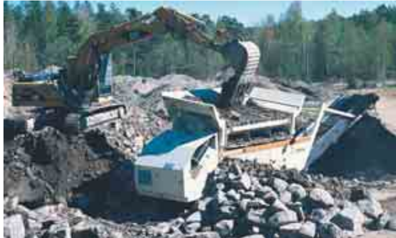
The adjustable speed, cassette style hopper conveyor is capable of moving a variety of different feed materials.
