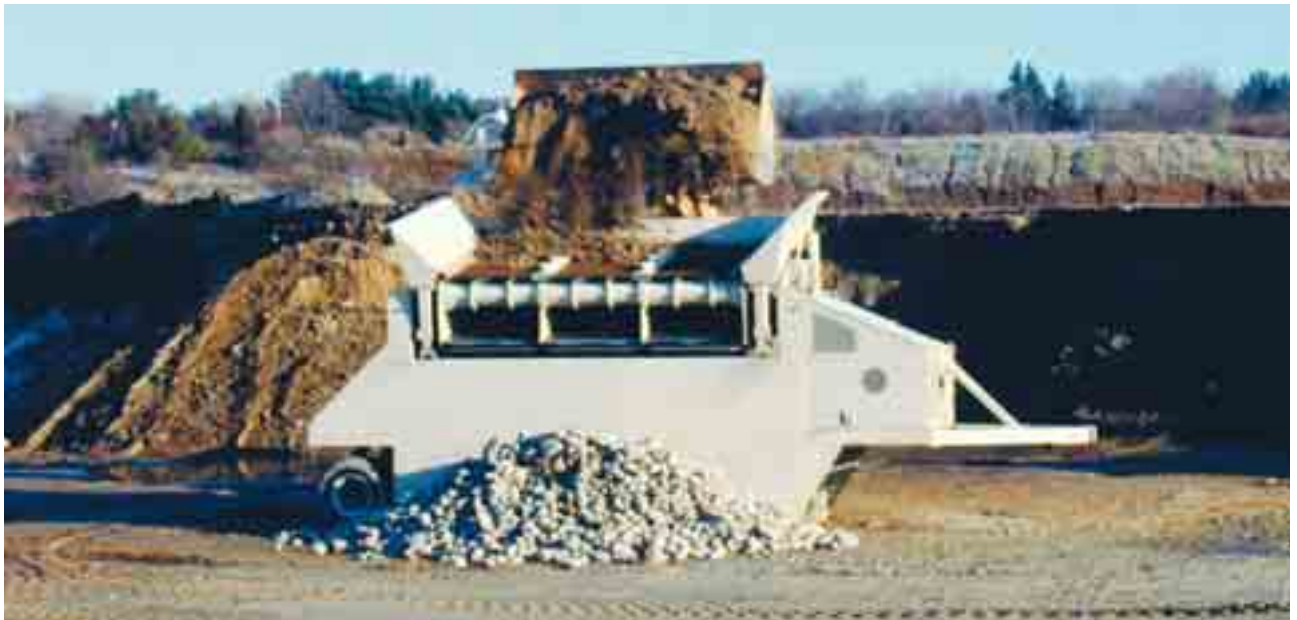
The convertible shakerhead of Nordberg CV100 adds versatility and productivity of the mobile screen.
