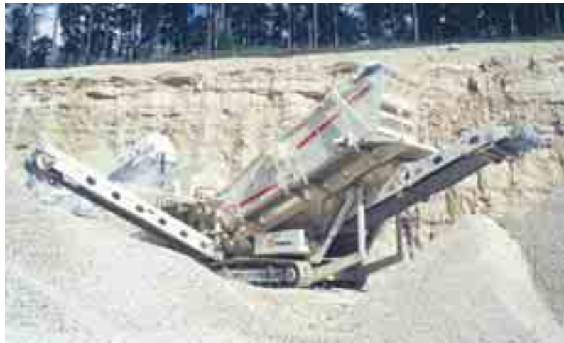
High screening capacities are ensured with efficient, triple-deck DS screen.
