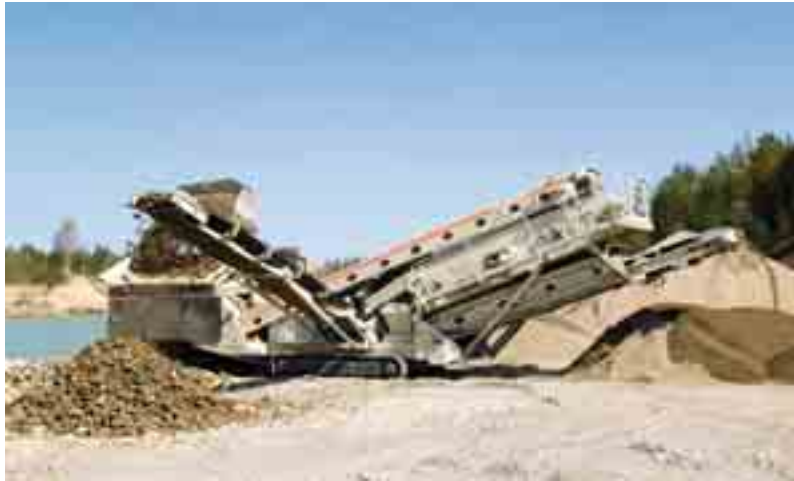
The standard unit Lokotrack ST358 mobile screen is capable of producing two accurately sized fractions.
