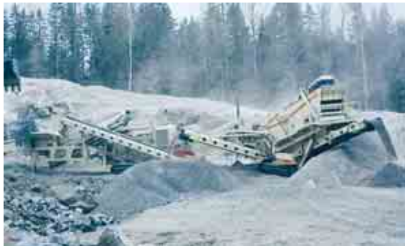
Lokotrack ST620 screening the output of an LT300HP mobile crushing plant for secondary crushing.
