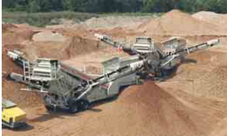
The maintenance platform provides easy access to the screen panels for screen mesh replacement.
