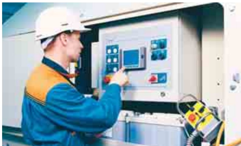
The Nordberg IC300 intelligent controller supervises and adjusts the ST171 automatically for optimum screening results.
