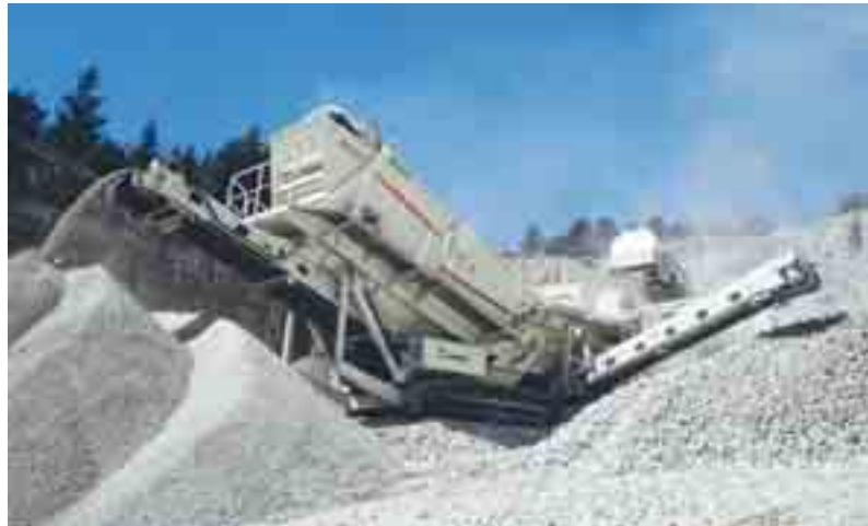
Full mobile crushing and screening process with Lokotrack LT1415 and ST620.
