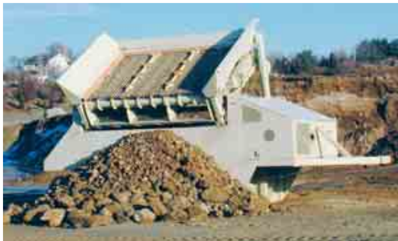
Remote controlled tipping cycle to clear the shakerhead of any [unwanted] debris is a standard feature on the Nordberg CV100 mobile screen.
