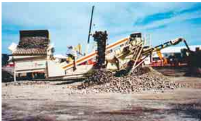
A hammermill type shredder and a remote control tipping agid function are available as options for SW348.
