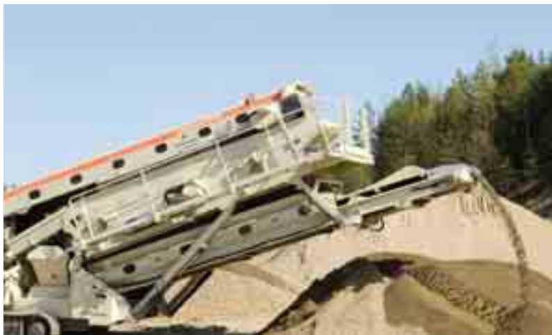
The ST358's end to end crowning screen is more efficient than similarly sized flat screens.
