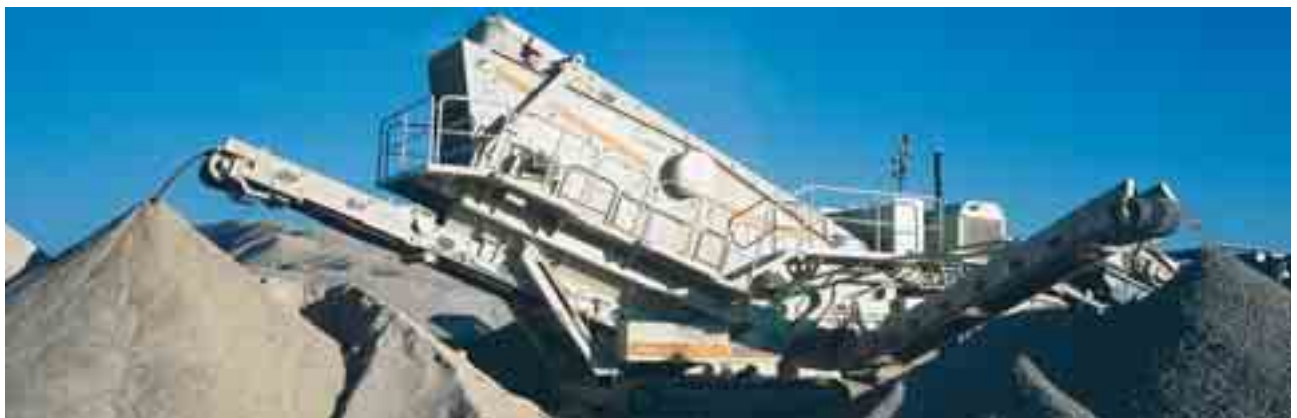
The triple-deck DS screen of Lokotrack ST620 is specially designed for mobile applications.
