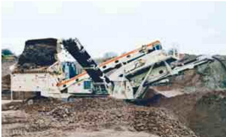
The hydraulically folding on-board stockpiling conveyors allow for fast set up times.
