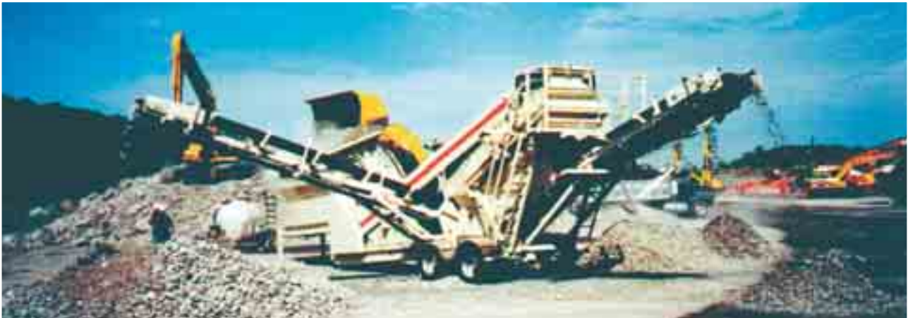
The Nordberg SW348 on-board stockpiling and product conveyors with fast set-up times eliminate the need for off plant stacking conveyors.
